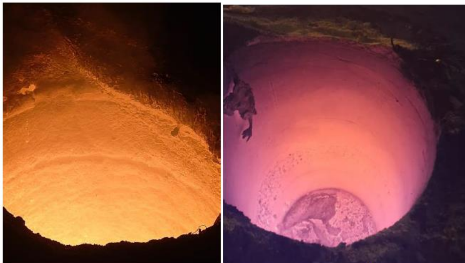
Fig.1: Kellundite MS 800 After 40 heats with millscale | Fig.2: K85 after sintering heat
