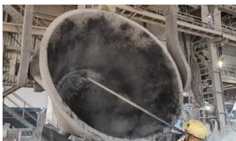
Fig. 1. Slag pot coating by graphite-silica solution
