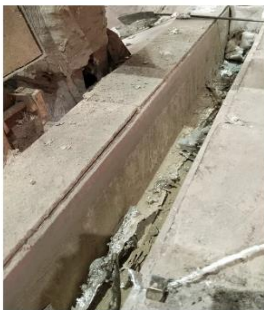
Fig. 1: Fused silica launder | Fig. 2: no sticking and no penetration of molten aluminum
